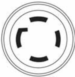
Figure 2-10: 120/240 VAC, 30 Amp Receptacle
